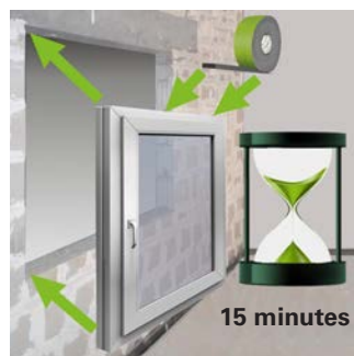
Figure 4: Install the window within 15 minutes.
