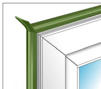
Fig 2 Form a 20 mm fold in the corner area
