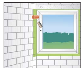
Fig 4 Consolidate the butyl bond using a roller
